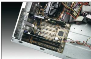
2.3 Locate an empty PCI expansion slot. It is usually white in color.
