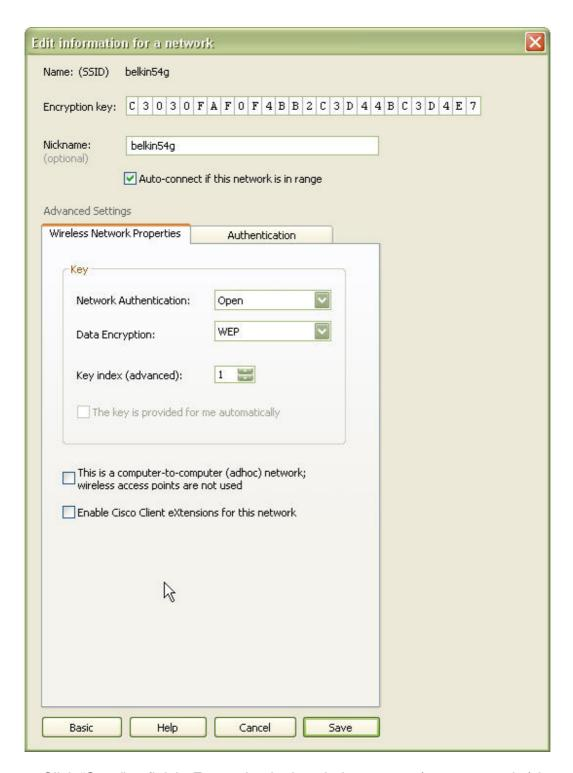
**3.** Click "Save" to finish. Encryption in the wireless router (or access point) is now set. Each of the computers on your wireless network will now need to be configured with the same security settings.
