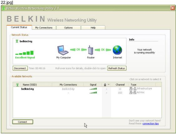
The WNU's default screen is the "Current Status" tab. The "Current Status" tab displays the current Network Status and Available Networks.
