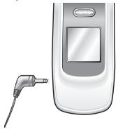
When the phone rings, press and hold the button on the ear-microphone for more than 1 second to answer the call.
