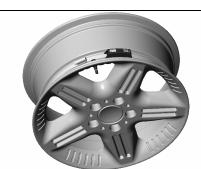
The base of the drop centre well must be flat and wide enough to allow the transmitter to contact the rim over its complete width.
