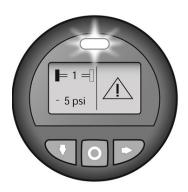
This alert is intended to give you an early indication that the tire is low/high. This alert is temperature typically based on the compensated value (if temperature compensation is selected for the alert). If so, you may see that the pressure is above the CIP, but due to the temperature of the tire, the pressure is actually low or high depending on the deviation value showed.
