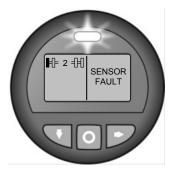
A Sensor Fault Alert will be issued for any programmed sensor for which the Receiver/ECU has not received data for a predetermined time. Typically, this time is set to 35 minutes. Sensor Fault Alerts are self-clearing as soon as data is received from the given sensor. Prolonged Sensor Fault Alerts can be an indicator of damaged or missing sensors and should be addressed to ensure the system is functioning properly. <u>Tires with active Sensor Faults cannot provide</u>
