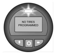
This message will be displayed after the startup sequence if the Receiver/ECU has not been programmed with any axle and wheel configurations. In this case the system is not functioning and no pressure or temperature alerts will be displayed. This should be reported to maintenance to be corrected as soon as possible.
