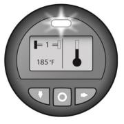
This alert is intended to give you an indication that the temperature of the air in the tire has reached a critical point and should be investigated.
