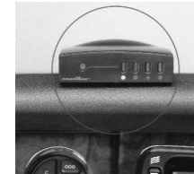
RECEIVER ATTACHED TO SURFACE WITH VELCRO® STRIPS
