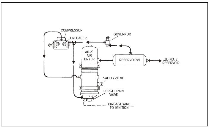
FIGURE 18 - TYPICAL INSTALLATION FOR THE AD-2™ AIR DRYER
