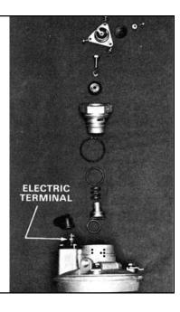
FIGURE 16 - AD-2™ AIR DRYER END COVER
