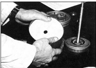
FIGURE 8 - ASSEMBLY OF DESICCANT CARTRIDGE
