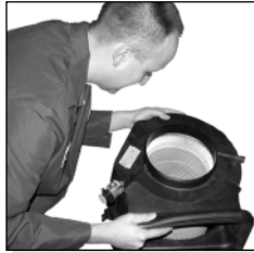
Inspect the engine air cleaner.
