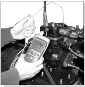
Testing the temperature at the discharge fitting.
