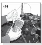
Testing the temperature at the discharge fitting.
