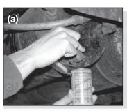
Drain <u>all</u> air tanks (reservoirs) into the Bendix<sup>®</sup> BASIC<sup>™</sup> test cup. (Bendix kit P/N 5013711).
