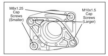
FIGURE 9 - REAR END COVER ATTACHMENT BOLTS
