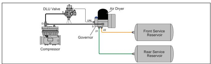
FIGURE 6 - TYPICAL 360 (DLU) COMPRESSOR AIR CHARGING SYSTEM
