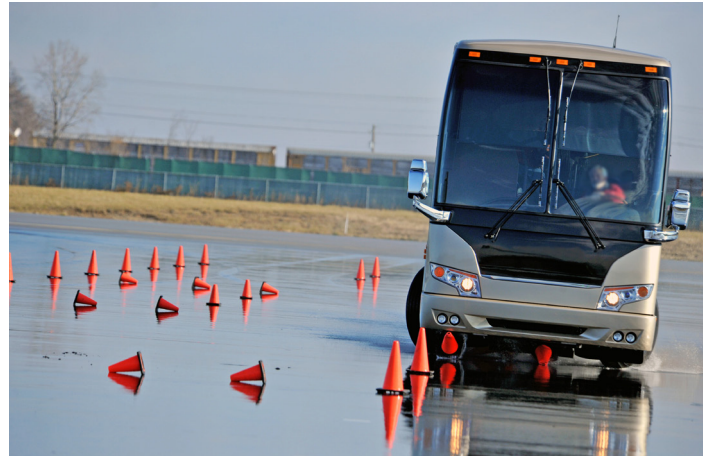
Above image shows a vehicle on a test track in a potential out-of-control scenario – on a slick surface (note the cones!)
