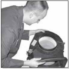
Inspect the engine air cleaner.
