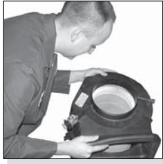
Inspect the engine air cleaner.
