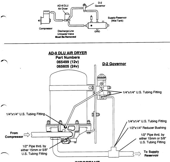
IMPORTANT: The Discharge Line Unloader Valve must be removed for the AD-9 DLU Air Dryer to function properly.
