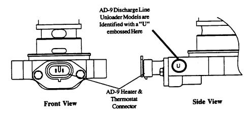
Partial view of the Purge Valve assembly for AD-9 for Discharge Line Unloader system
