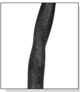
Partly collapsed inlet line shown.
