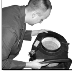
Inspect the engine air cleaner.
