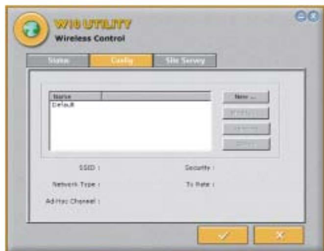
In the beginning, there is no default settings. A new WLAN setting profile can be set up by press “New” and one configuration menu will pop up.
