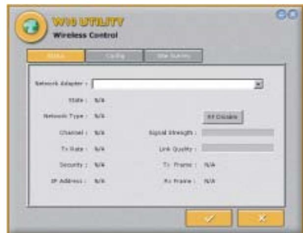
In “Scanning” state, it means that the node cannot detect the SSID to an access point within range and is searching for an available access point. Also, if the driver failed to initiate for some unknown reasons, this field will display an error message.
