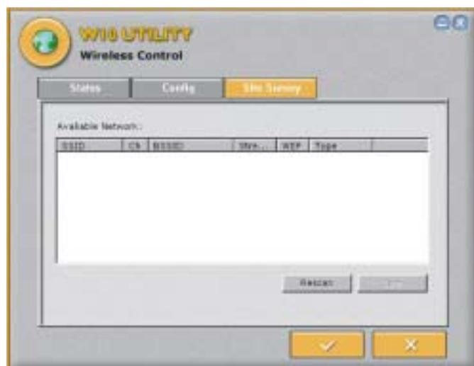
and then list their SSID, channel, BSSID and signal respectively.
