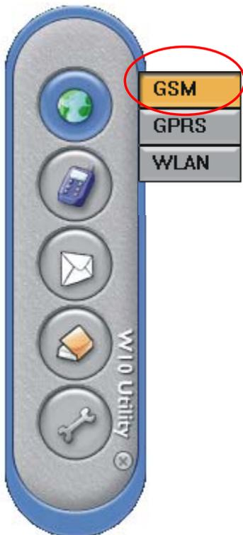
When users choose network configuration, the submenu will pop up. Left click the mouse on the GSM item and the GSM control panel will pop up.
