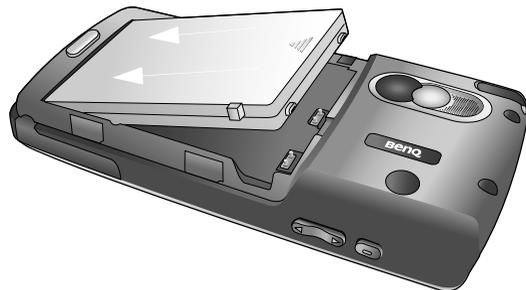
3. Push the battery against the top of P31 to insert the teeth into the holes, then press the battery down gently to click it back into place.
