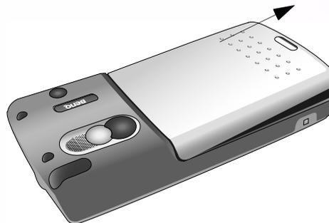
3. Slide the battery latch backward and lift the battery upward.
