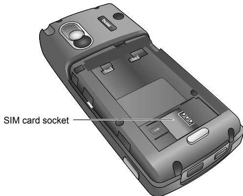
2. Slide the SIM card in under the metal plate in the SIM card slot with the SIM card's metal contacts facing down and the cut corner at the bottom right.
