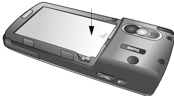
4. Push the battery door down on the phone and slide it into place.
