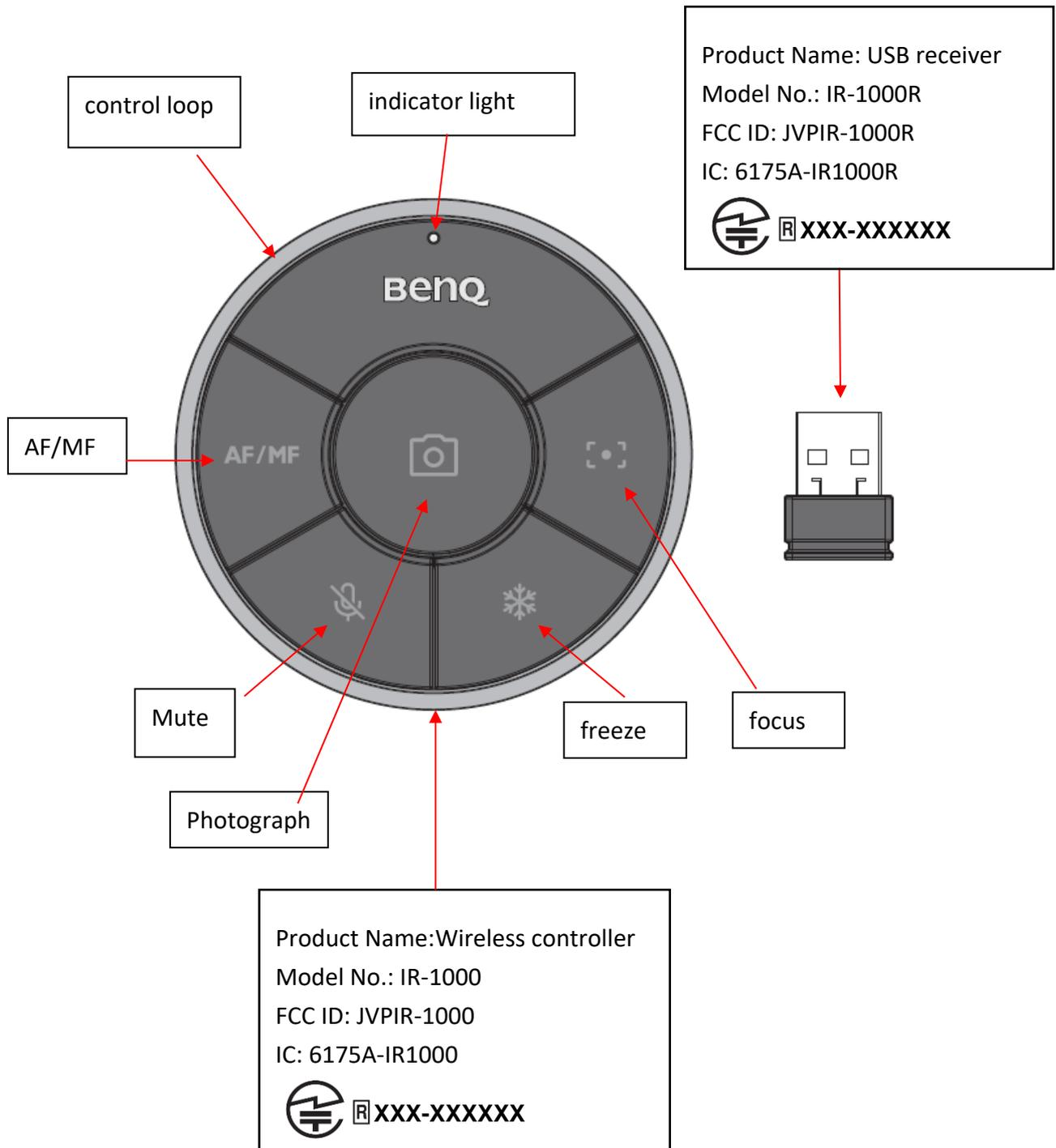
1. Indicator light--Lights up white when the controller is being operated, and flashes red after being operated when the battery is low.
