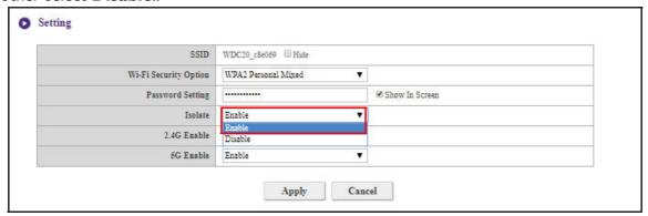
You can choose the available frequencies for the Host's Wi-Fi signal in the **2.4G Enable** and **5G Enable** fields. A 2.4G Wi-Fi signal is a signal that features a larger coverage range but slower data speeds and is more commonly used by older mobile devices, while a 5G Wi-Fi signal features faster data speeds at a smaller range. To enable or disable either 2.4G or 5G Wi-Fi signals by selecting **Enable** or **Disable** in the **2.4G Enable** and/or **5G Enable** fields.
