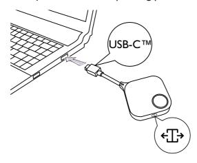
2. When the Button is successfully connected to the laptop, the LED indicator of the Button will blink green.
