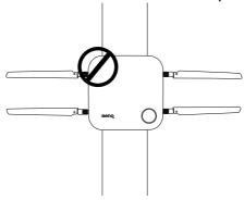
• If the Host is attached to a metallic ceiling mount ensure that the antennas are at least 3 cm away from the metal portion of the ceiling mount:
