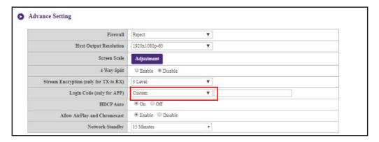
**HDCP Auto** is a security setting that allows you configure whether or not HDCP digital copy protection is automatically enabled for the content output by the Host. The default setting for this field is **On**, which means that HDCP copy protection will be automatically enabled by Host for content that features HDCP copy protection and disabled for content that does not feature HDCP copy protection. To change the setting so that HDCP copy protection is always enabled by Host select **Off**.
