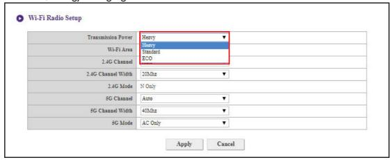
In the **2.4G Channel** and **5G Channel** fields you can configure the Host to automatically select the wireless channel with the best performance for either signal during the initial setup of the Host by selecting **Auto**, or you can select a wireless channel manually. The default **2.4G Channel** and **5G Channel** setting for the Host is **Auto**.
