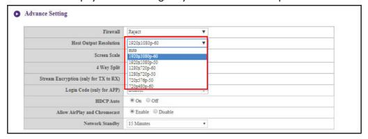
**Screen Scale** allows users to adjust the borders of the Host's video output so that it properly fits the screen of the connected display. This setting is mainly intended for users who connect the Host to a touchscreen display, so that the edges of the video align to the edges of the display's screen to ensure the accuracy of touch gestures. To adjust the **Screen Scale** setting, click the **Adjustment** button, then use the toggle buttons to scale the video to fit the screen.
