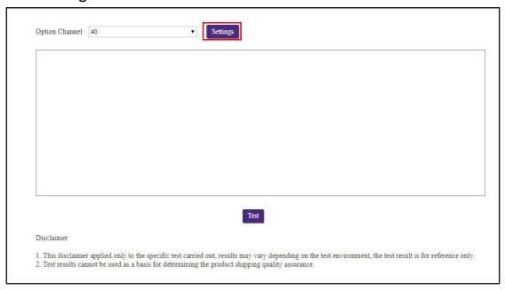
3. Click the **Test** button. The results of the test will be shown in the main window.
