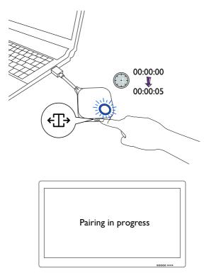
7. The LED indicator of the Button will turn static green when the Host and Button are successfully paired.
