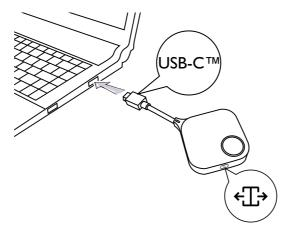
2. When the new Button is connected to the laptop, the LED indicator of the Button will flash red. The Button is in pairing mode, waiting to pair with your Host.
