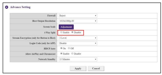
**Stream Encryption** is a security setting that allows you to select the level of encryption for the connection between the Host and Buttons in order to protect it from hacking. The default setting for this field is **3 Level**, to change the setting to a lower level of encryption select **2 Level**.
