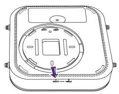
4. Attach the rubber feet to the recesses on the lid and put the Host right next to the display.
