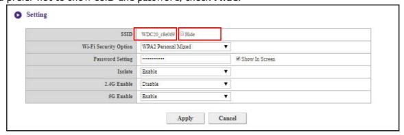
Wi-Fi Security Option provides the user WPA2 Personal and WPA2 Personal Mixed security options for the Host's wireless connection when users access the web management interface via a wireless network.
