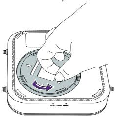
3. When the lid is correctly installed on the Host the alignment hole on the lid should be pointed to the **LOCK** print at the front side of the Host.
