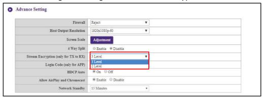
**Login Code** allows you to set a login password for connections by mobile devices which will appear on the guide screen. The default setting for this field is **Disable** which means that no login password is needed for mobile devices to connect to the Host. To set a custom login password for mobile devices, select **Custom** and then enter the password you want in the field to the right of the **Login Code** field. To set an automatically generated login password select **Random**.
