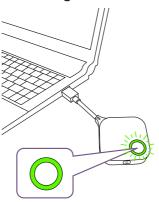
4. When the Button is ready to present, the LED indicator will turn solid green. Press the Present key when the LED indicator turns green.
