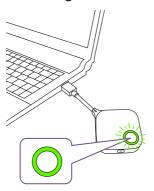
3. When the Button is ready to present, the LED indicator will turn solid green. Press the Present key when the LED indicator turns green.
