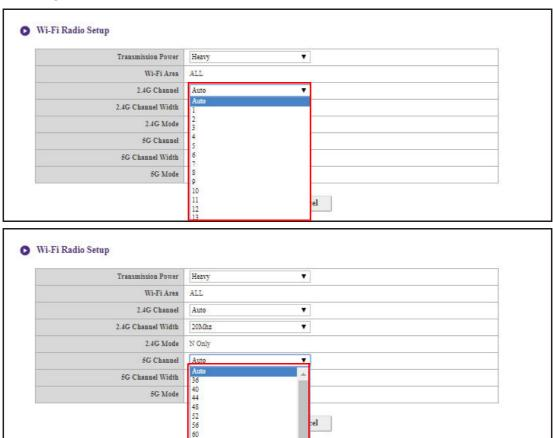
In the **2.4G Channel Width** and **5G Channel Width** fields you can configure the channel width for your 2.4G and/or 5G Wi-Fi signal. The available options for **2.4G Channel Width** are **20MHz** and **40MHz**, while the available options for **5G Channel Width** are **20MHz**, **40MHz**, and **80MHz**. The default channel width for **2.4G Channel** is **20MHz** while the default channel width for **5G Channel** is **40MHz**.
