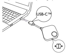
3. The LED indicator of the Button will flash green while the Button is starting up.
