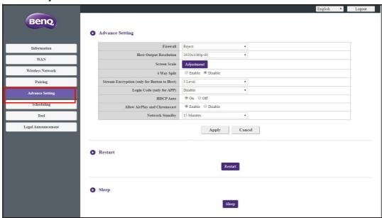
**Firewall** is a security setting that allows you to block/reject users from accessing the Host via its WAN port in order to protect it from hacking. The default setting for this field is **Reject** which enables the firewall and rejects access to the Host via its WAN port. To disable the firewall and allow devices to access the Host via its WAN port select **Accept**. A warning message is prompted to let you know the security risk.
