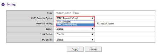
**WPA2 Personal** allows only users with Advanced Encryption Standard (AES) encryption to connect to the Host.
