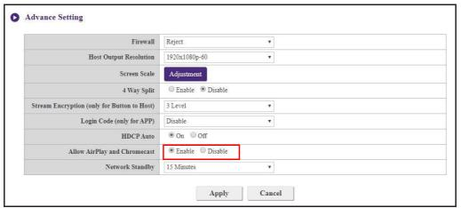
**Network Standby** allows you to set the time of inactivity before the Host enters network standby mode.
