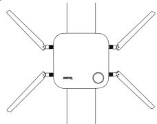
• Avoid positioning the antennas in a horizontal manner, this may result in a weak signal reception:
