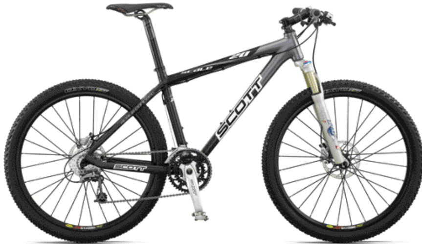
XC Elite racing | frame CR1 carbon technology | front FOX F 80FRL, Lockout, 80 mm | Shimano XTR/XT 27 speed, DT Swiss/Mavic wheelset, Shimano XT disc brakes | 10 kg (22 lbs)
