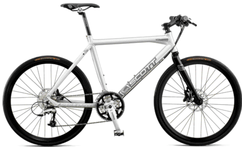
SUB 10 Fast city/commuting bike | frame aero shaped 6061 alloy, hydroformed tubing, semi-integrated headset, Evo dropout | Shimano XT/LX/Deore 27 speed | 26" wheels available
