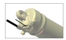
2 Insert a new cable via lever hole and cable housing and push it into the shock as shown around the remote wheel (S6)
