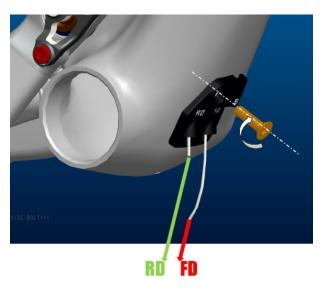
Push the outer cable housings on the cables into the cable guide but make sure to respect the needed length as shown in the next drawing!
