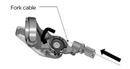
and secure the cable by fixing the 2mm allen screw with a tightening torque of 0.9Nm/ 8lb/in as shown on the drawing below on the roll.
