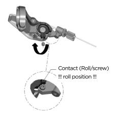
Cut the cable 5mm behind the roll and secure it with a cable end-cap.
