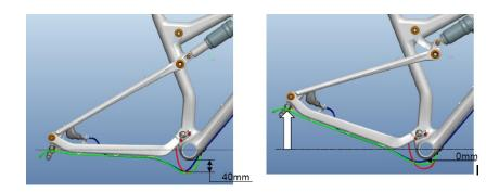
For the rear brake please assemble the cable as shown in the following drawings:
