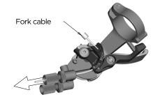
Fix the cable with the 2mm allen screw on the barrel adjuster on the fork crown with a tightening torque of 0.9Nm/ 8lb/in, cut the cable and secure it with a cable end-cap. Please refer for this action also to the manual of SRAM/RockShox attached to the bike.
