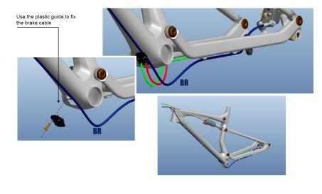
The cable guide can be ordered via the Scott distribution with parts number:
