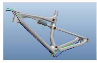
The carbon frames of Spark have an internal shifting cable routing with cable stops on the front end of the downtube as shown in the drawing below.
