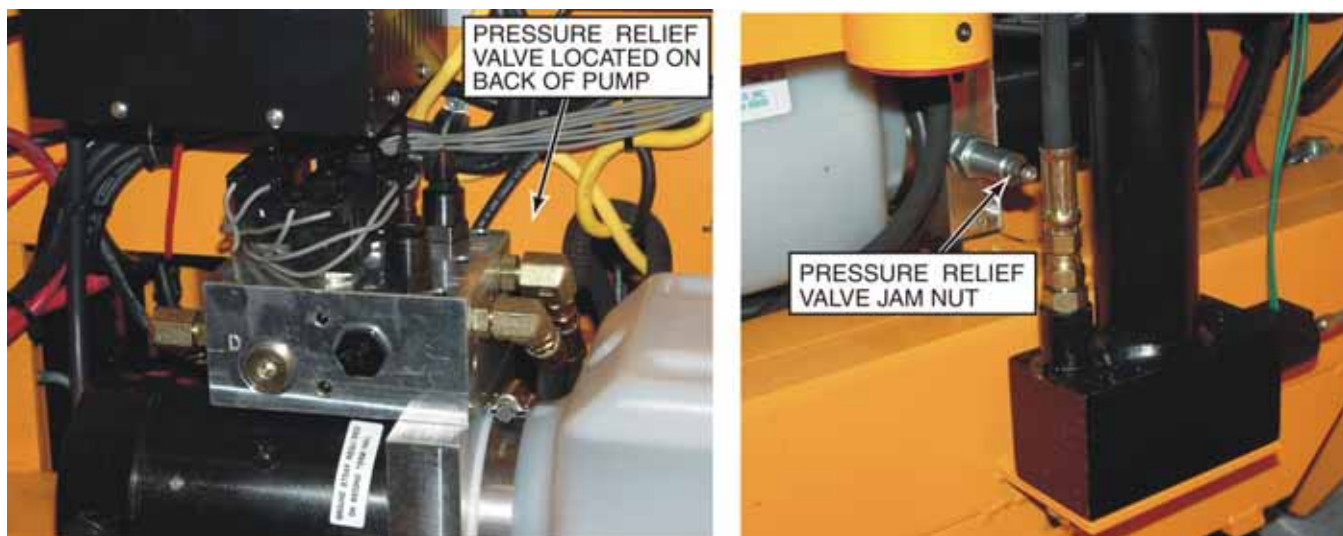
Figure 4-6. Pressure Relief Valve Adjustment
