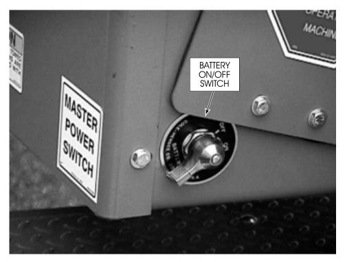
Figure 3-1. Battery ON/OFF Switch
