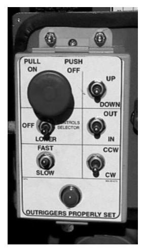
Figure 3-2. Lower Control Panel (DC Model)
