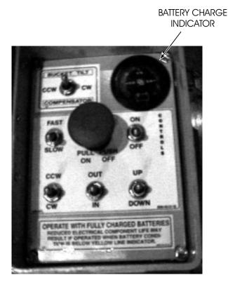
Figure 3-3. Upper Control Panel (DC Model)
