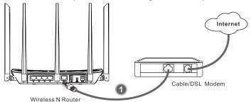
2 Connect your computer to the Port labeled 1~4 on the Router with an Ethernet cable.
