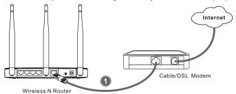
Connect your computer to the Port labeled 1~4 on the Router with an Ethernet cable.
