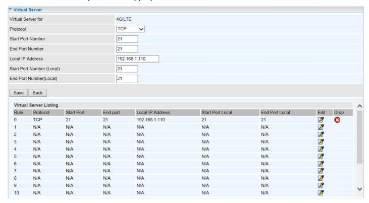
**Virtual Server for:** Indicate the related WAN interface to allow outside network to communicate with the internal LAN device.
