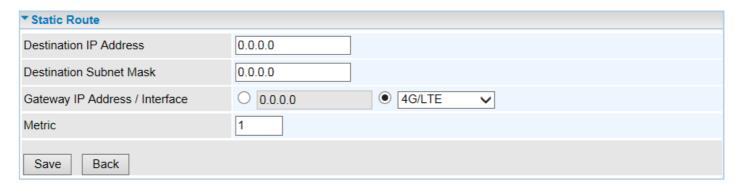
**Destination IP Address:** This is the destination subnet IP address.
