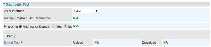
Ping other IP Address: Click Yes to ping any desired IP address or a domain.
