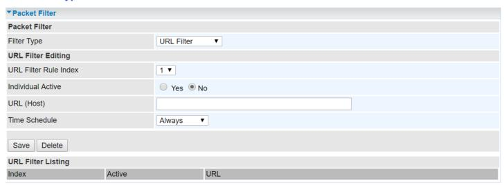
**URL Filter:** Select **Activated** to enable URL Filter. **URL Filter Rule Index:** The numeric rule indicator.
