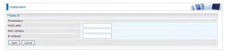
Enter the MAC Address, IP Address, and then click Apply to confirm your settings. But the IP assigned should be outside the range of 192.168.1.100-192.168.1.199.
