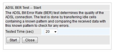
Select the Tested Time (sec), press Start to start test.
