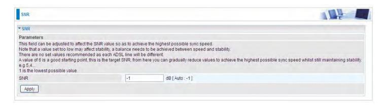
SNR: Change the value to adjust the DSL link rate, more suitable for an advanced user.
