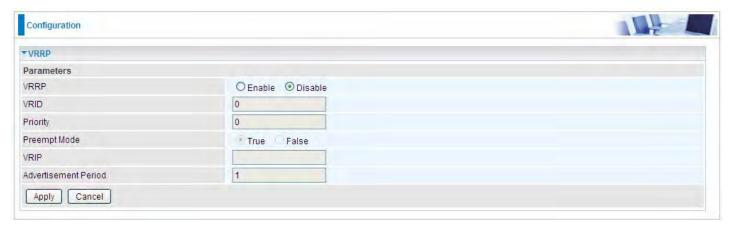
VRRP: Check Enable radio button to activate this function. The default setting is "Disable".
