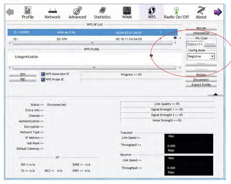
3. The router's (AP's) SSID and security setting will now be configured to match the SSID and security setting of the registrar.
