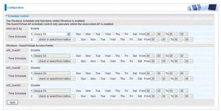
**Time Schedule:** Set when the SSID works. If user wants the SSID works all the time, please select "Always On"; if not, please set or select the exact time your want the SSID works. Here user can set two separate intervals.
