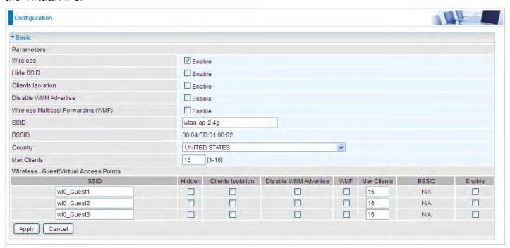
Wireless: Default setting is set to Enable. If you do not have any wireless devices, check the checkbox again to unselect.
