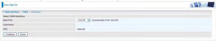
2. Select the 3G/LTE mode, and enter the APN, username, password from your ISP; and check with your ISP with the authentication method setting for each SIM (SIM1 and SIM2).
