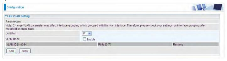
**LAN Port:** Select the LAN port users want to set LAN VLAN. **VLAN Mode:** Check if to enable LAN VLAN for the select port.
