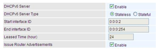
With this method, the PCs' addresses in LAN are configured like above method, but they can obtain such information like DNS from DHCPv6 Server.
