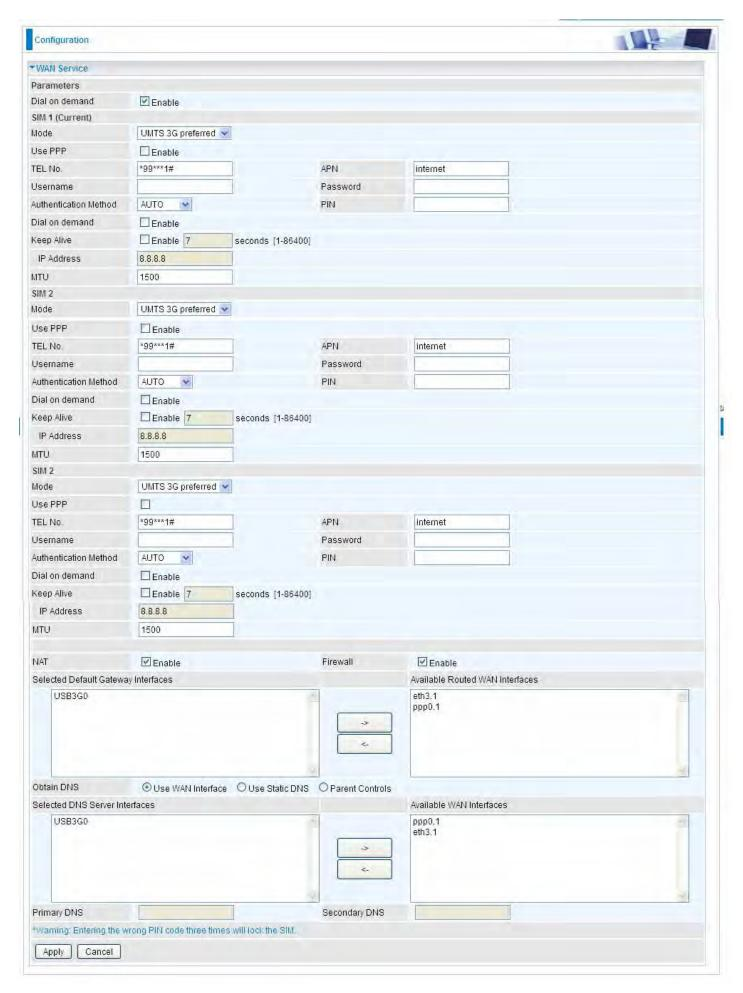
**Dial on demand:** If enabled, the 3G/LTE will work in dial on demand and be brought up only when there is no active default route. In this mode, 3G/LTE work as a backup for the WAN connectivity. While if disabled, 3G/LTE serves as a normal interface, and can only be brought up when it has
