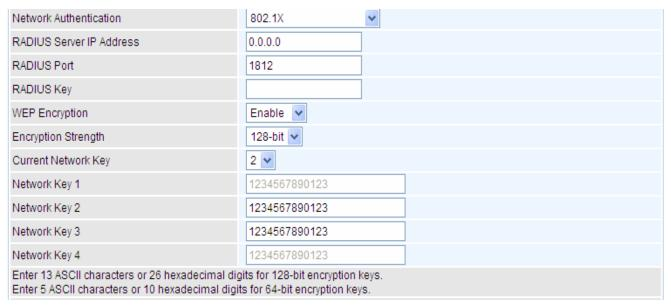
**RADIUS Server IP Address:** RADIUS( Remote Authentication Dial In User Service), Enter the IP address of RADIUS authentication server.
