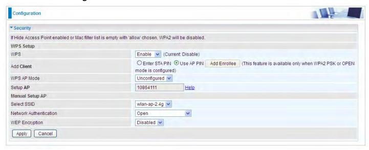
2. Launch the wireless client's WPS utility (eg. Ralink Utility). Set the Config Mode as **Registrar**. Enter the **PIN** number (10864111 (device) for example) in the PIN Code column then choose the correct AP (eg. wlan-ap-2.4g) from the WPS AP List section before pressing the PIN button to run the scan.
