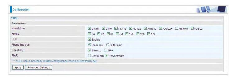
**Modulation:** There are 8 modes "G.Dmt", "G.lite", "T1.413", "ADSL2", "AnnexL", "ADSL2+", "AnnexM" "VDSL2"that user can select for this connection.
