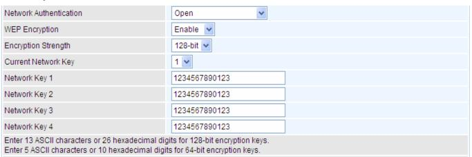
**WEP Encryption:** Select to enable or disable WEP Encryption. Here select Enable.
