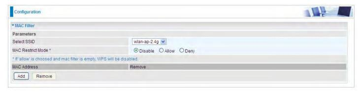
**Select SSID:** Select the SSID you want this filter applies to.
