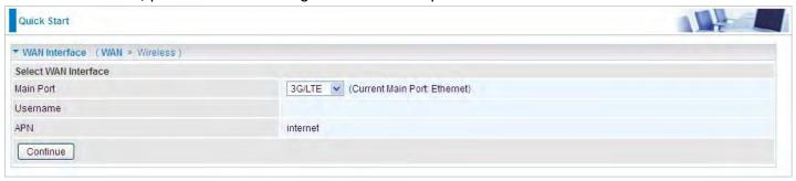
2. Select the 3G/LTE mode, and enter the APN, username, password from your ISP; and check with your ISP with the authentication method setting for each SIM (SIM1 and SIM2).
