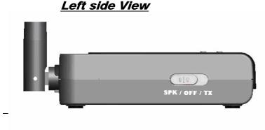
SPK ---- Speaker mode TX ---- Transmitter mode OFF ---- Power off
