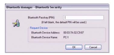
• The window in which you enter the passkey will not appear once you have connected more than two times to the device.
