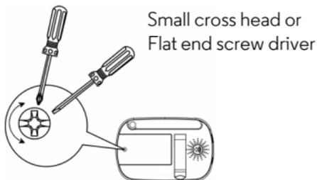
2. Replace the battery cover over the compartment and gently tighten the screw in a clockwise direction using a Small cross head or Flat end screw drivers.
