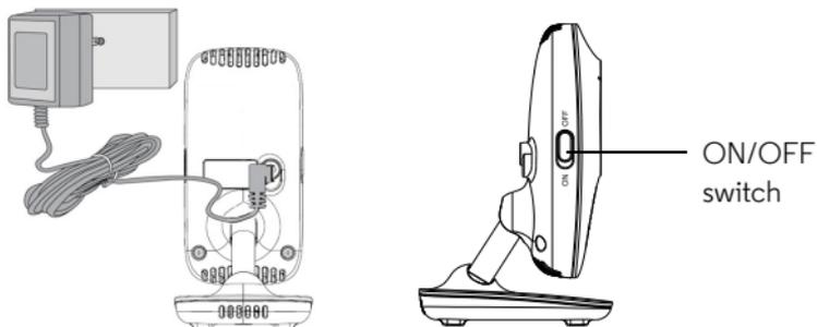
1. Connect the power adapter to an electrical outlet and insert the plug into the DC power socket on the back of the Baby Unit (Camera).
