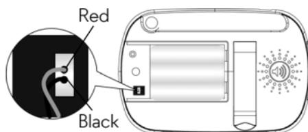
1. Insert the wire tab of the rechargeable battery pack into the contact slot as shown above and fit the battery pack into the compartment.
