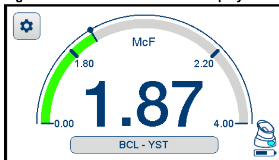
Figure 29: VITEK® DensiCHEK® Display Base Screen - YST and BCL
