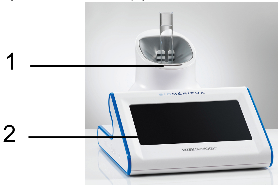
Figure 17: VITEK® DensiCHEK® Display Base with the Pod
