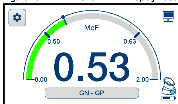
Figure 28: VITEK® DensiCHEK® Display Base Screen - GN and GP
