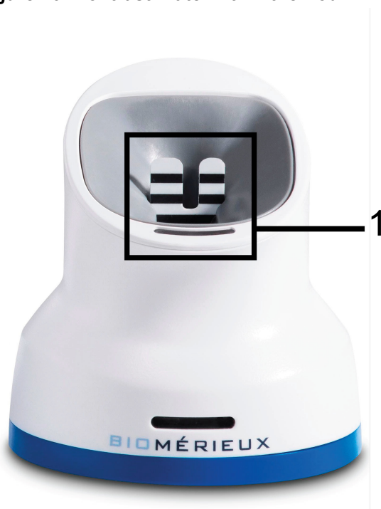
Figure 16: Contrast Plate Within the Pod
