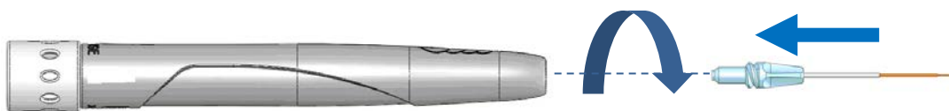
Figure 2.7: Insert the fiber tip into the handpiece and twist clockwise until snug
