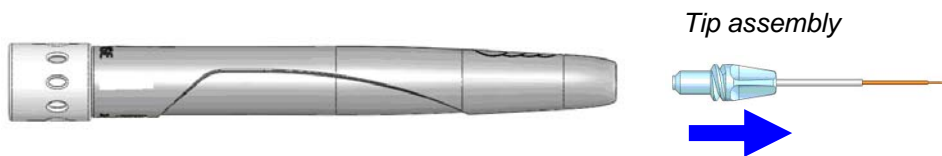
Figure 18: Disconnecting the fiber Tip (twist first counter clockwise)
