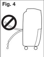
**NOTE: To help prevent leakage, you should use a marker to denote the location where the hose meets the housing on the rear of the unit. Periodically check to make sure this indicator has not moved away from the housing to ensure that your hose will not leak.** Leakage inside the unit will fall into the water reservoir. If this happens you can empty the water reservoir by following the instructions above in the "Emptying the Water Reservoir" section.
