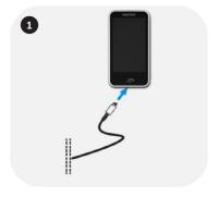
1. Connect the micro-USB plug of the charging cable to the mircro-USB input of the receiver (HR310).
