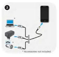
Connect the USB plug to the USB port of the AC power adapter supplied with your system, and connect the adapter to the power source. Alternatively, connect plug to the USB port of your computer or USB car charger adapter.
