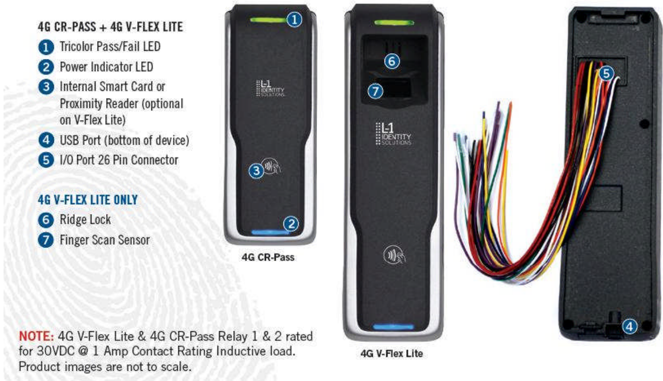
Figure 1-1 4G V-Flex Lite & CR-Pass
