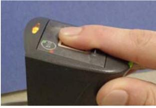
**Figure 18: Position Finger on Sensor**
