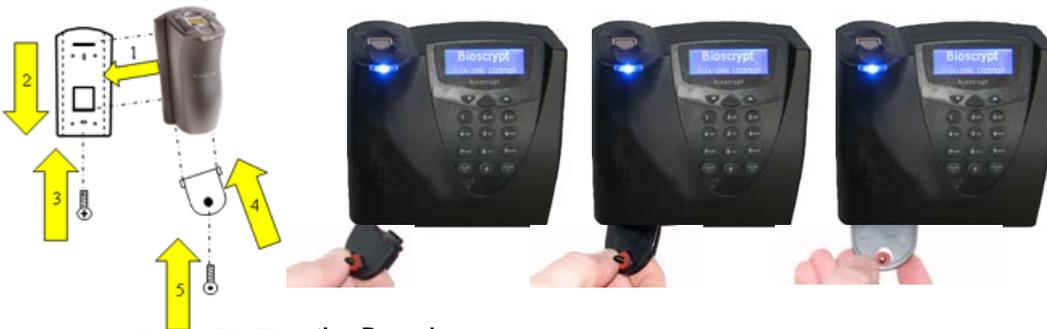
Figure 11: Mounting Procedures
