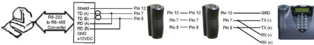
Figure 14: Wiring Diagram for RS-232 to RS-485 Converter
