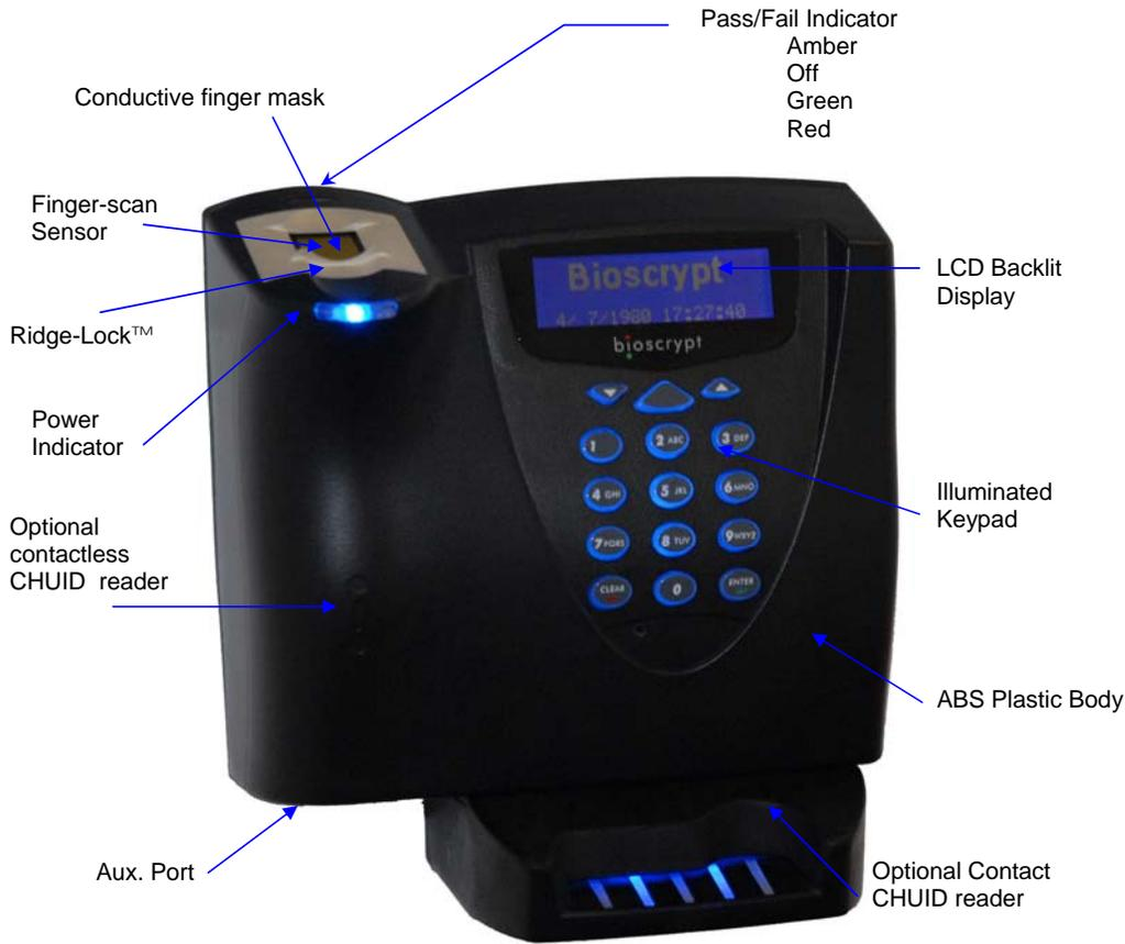
**Figure 2: PIV-Station (shown with Optional Contact CHUID reader)**
