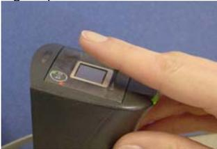
**Figure 21: Lift Finger Up and Off Sensor**
