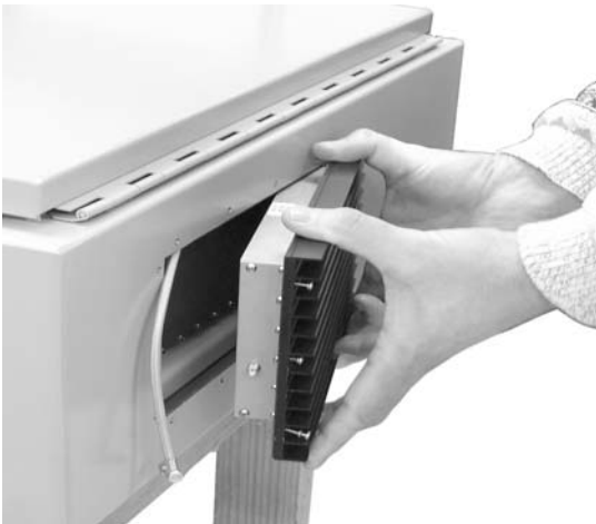
Figure 11: Slide amplifier towards bottom of cabinet to remove upper cable.
