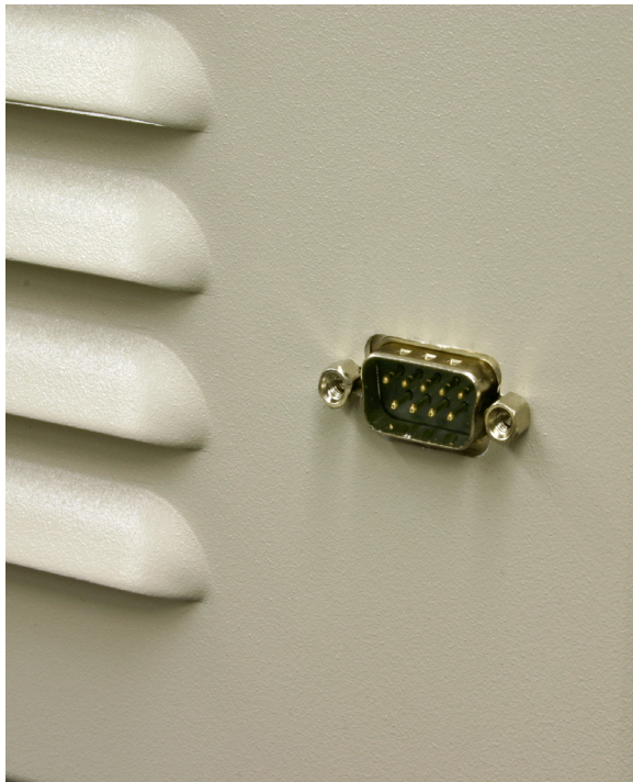
Figure 7: Remote alarm sensing connector.
