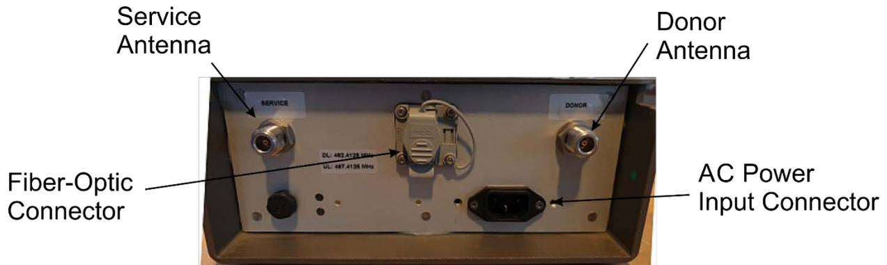
Figure 2. Connections on the DMR604
