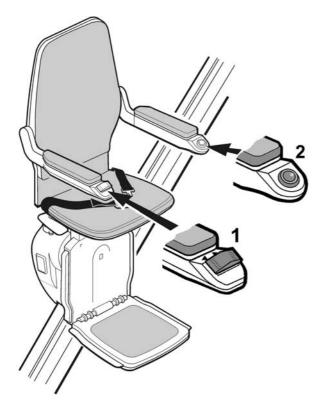
Your Stairlift is switched on and off using the On/Off Holding Switch (2).
