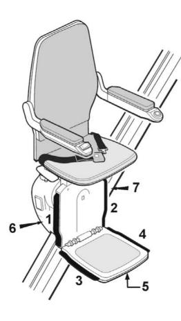
Before operating your Stairlift, ensure that there are no obstructions on the staircase. The Stairlift is fitted with seven safety edges:
