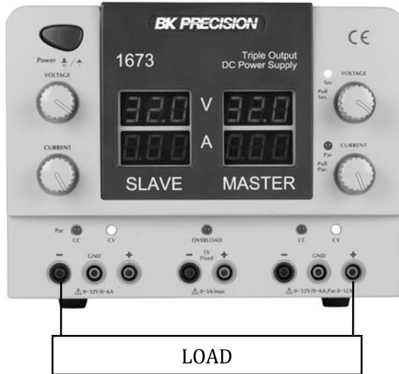
Figure 5 – Series Tracking Mode Load Connection
