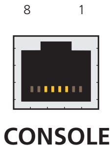
Figure 3-6. View of the console port on the SmartPath AP (LWN602HA).
