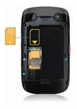
Slide the SIM card into the slot.
