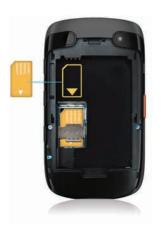
Slide the SIM card into the slot.
