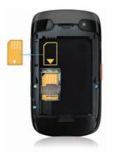
Slide the SIM card into the slot.
