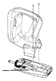
Ensure retaining screws go straight into the slots on the mobile computer.
