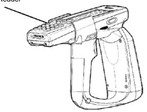
3. Attach two retaining screws. Ensure that they go straight into the mobile computer openings.
