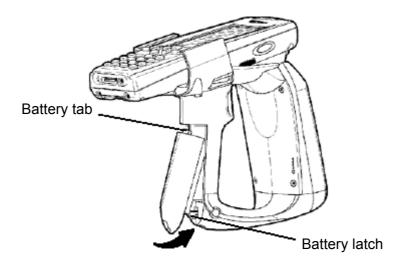
2. To **remove** the battery pack, push the battery release latch forward and remove the battery pack from the handle.
