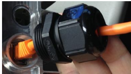
Figure 25 Ethernet Connector Encased in Environmental Housing
