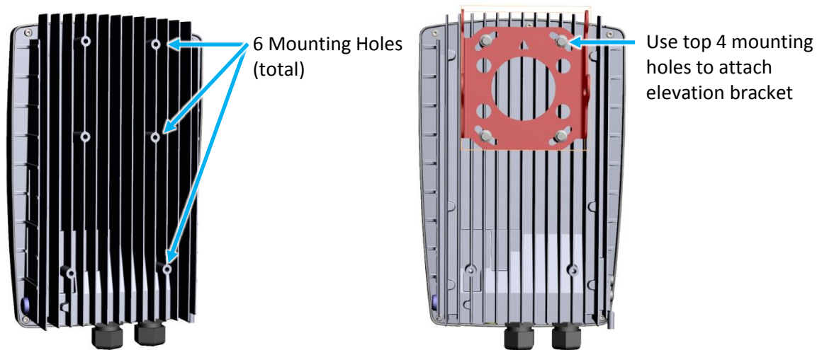
Figure 11 Attaching Elevation Bracket to Back of Module
