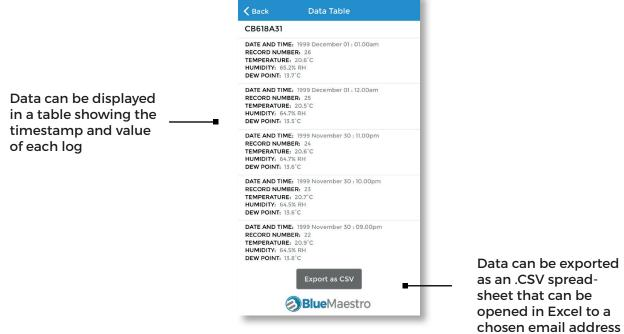
Once data has been downloaded from the Device into the iOS smartphone or tablet, the logged data can be graphed or viewed as a table. Both the graphs and the data table can be exported directly from the iOS smartphone or tablet via email to an email address.
