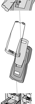
10. Insert the *Pager* into the *Charger* and fully charge the battery.
