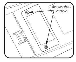
2) Use a phillips screwdriver to remove the two screws holding the cover plate in place.
