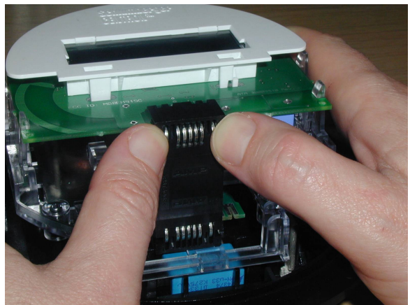
Figure 9: Board-to-board connector: TOP
